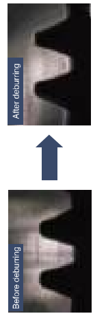
XEBEC product used/A31-CB25M Rotation speed:5500mm 2 /min Depth of cut:1mm Processing time:N/A Feed:2500mm/min
