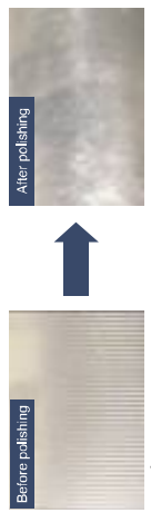
XEBEC product used/A21-CB25M Rotation speed:3500mm 2 /min Depth of cut:0.6mm Processing time:N/A Feed:100mm/min
